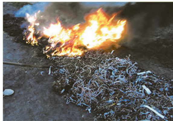
Open burning of electric wires for retrieval of copper in an e-waste processing village (Bui Dau, Vietnam)
