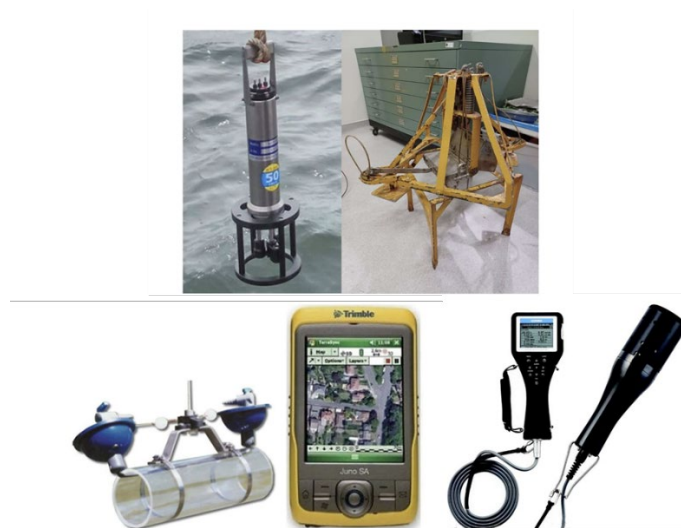
Figure.2. Survey Instruments i.e. Rinko CTD profiler, Smith-McTear grab sampler, Van Dorn water sampler, GPS Handheld and Water Quality Checker-Horiba
